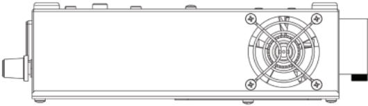
Upside down mounting - fixed to underside of shelf.
